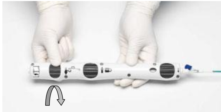
Figure 4.12: Rotating the Release Knob to Decouple the Implant from the Handle Assembly
